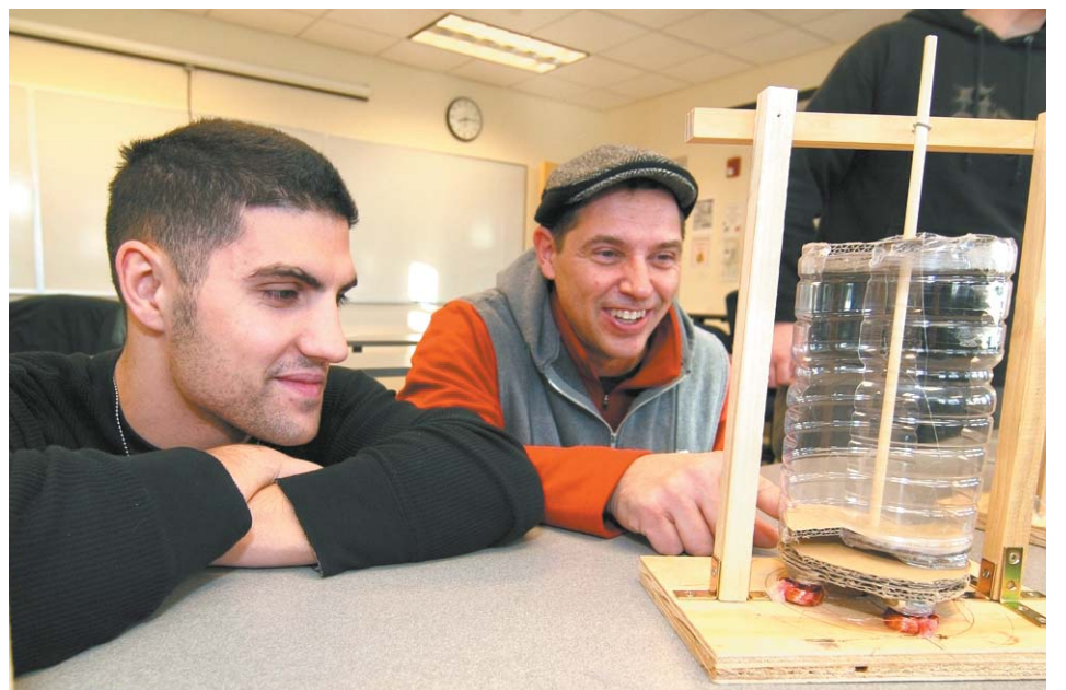
Justin Grasso of Andover examines the Savonius turbine he created with Professor Chanley of Wakefield.
